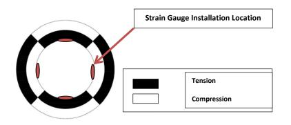
Figure 1- Stress/strain distribution along the pipe section loaded per ASTM C497 (D-Load) test and strain gauges installation location.
