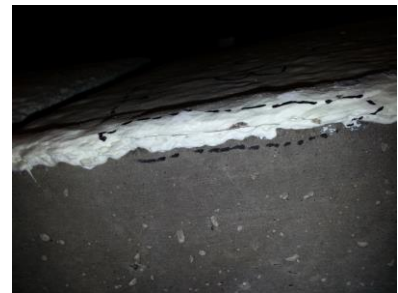
b) Type II failures with delamination expressed at edge of specimen.
