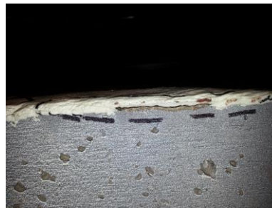
b) Type II failures with delamination expressed at edge of specimen.
