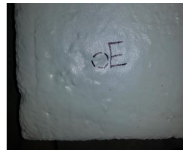
d) Type IV blow out failure.
