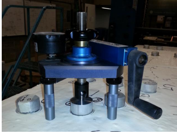
Figure 9 Dyna Z-15 pull-off test apparatus.
