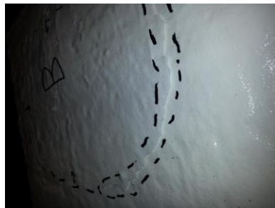
a) Type I punching shear failure
