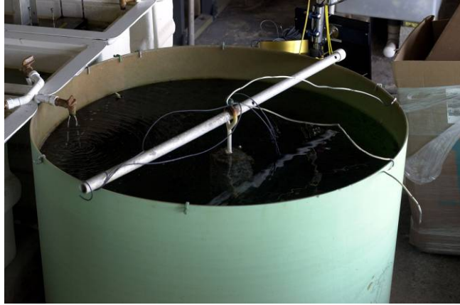
Figure 10 - Cathodic disbondment test tank with anode
