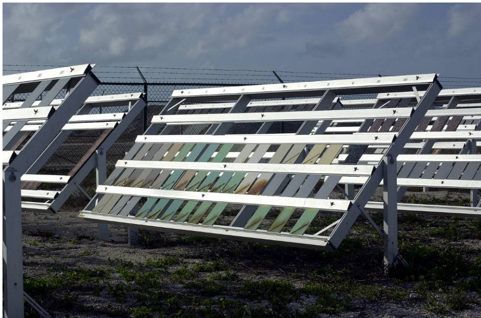
Figure 12 - Atmospheric exposure rack in Key West, Florida
