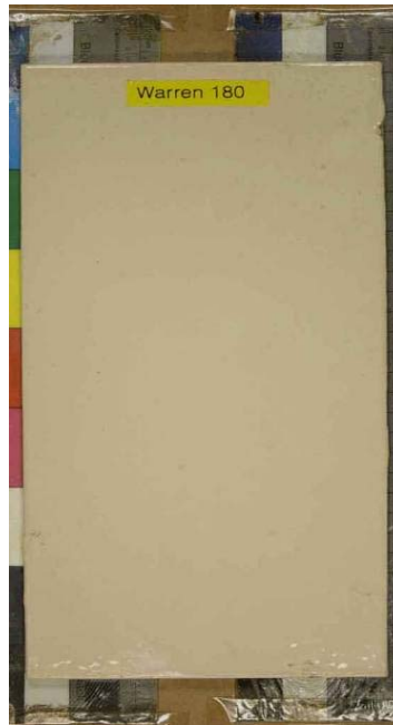
Figure 23 - Warren S-301 simulate boiler feed test panel
