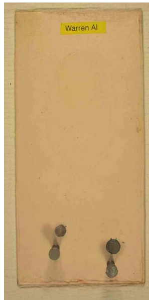
Figure 17 - Representative panels from alternate immersion testing
