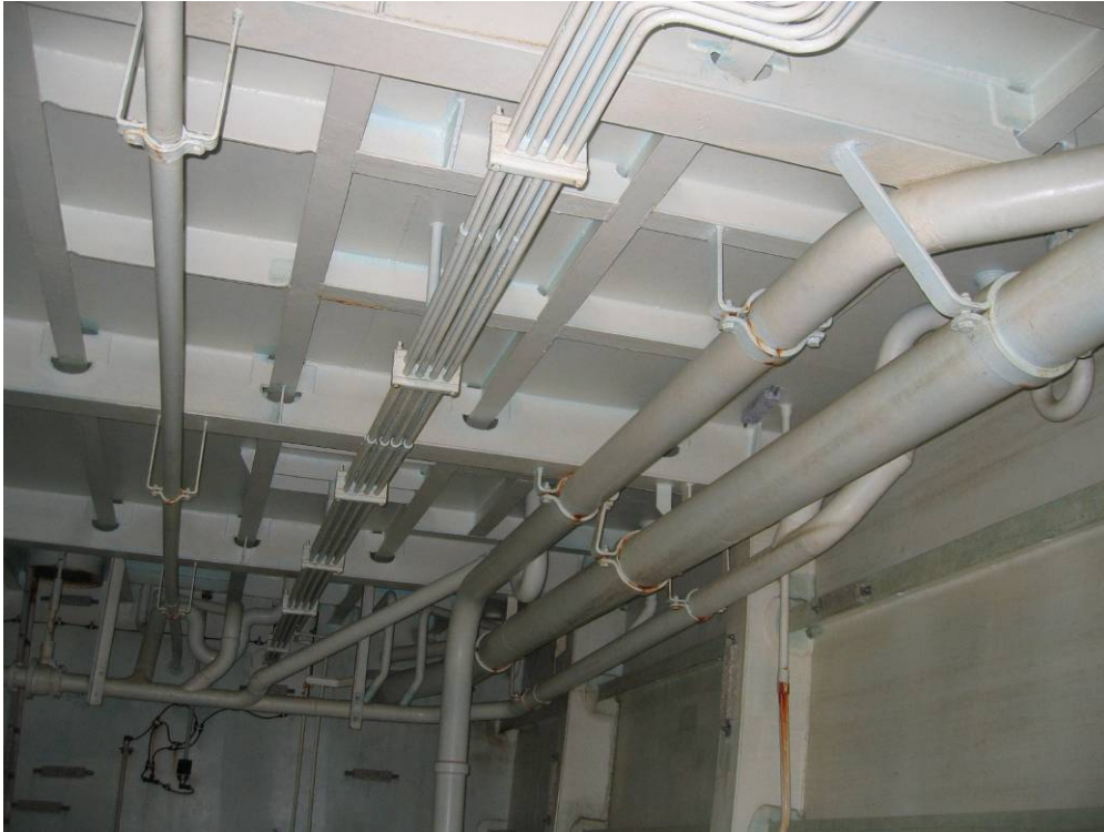
USS Oak Hill LSD-51 SWB Tk 3-121-1-W with Warren Environmental S-301 Rapid Cure coating system applied 15-months earlier. Looking Forward at the Overhead. All corrosion seen is rust stain originating from interior of pipe brackets.
