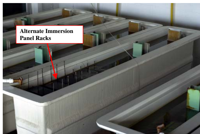
Figure 9 - Alternate immersion test immersion tanks
