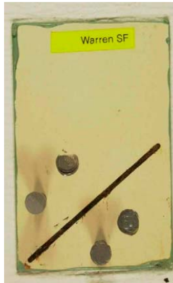
Figure 16 - Representative panel after 1000 hour B-117 test
