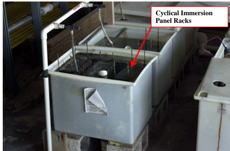
Figure 11 - Immersion tank used for cyclical testing
