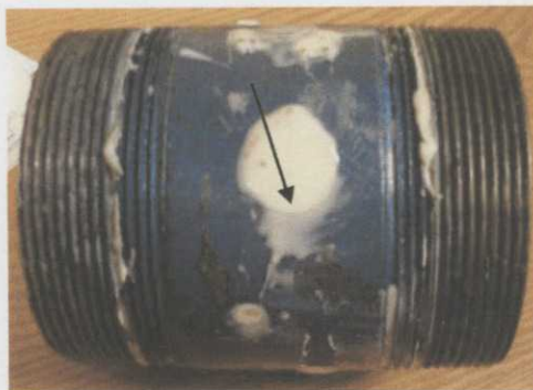
(a) following initial test to 2500 psi showing hairline crack around edge of \frac{3}{4} in. hole
